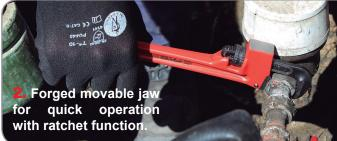
3. Graduations on hook jaw show approximate size of opening for different pipe sizes.
