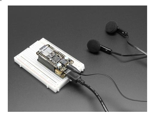
Bend all audio files to your will with the Adafruit Music Maker FeatherWing! It's a fun-size version of our Music Maker shield for Arduino (https://adafru.it/tbM)! This powerful shield features the VS1053, an encoding/decoding (codec) chip that can decode a wide variety of audio formats such as MP3, AAC, Ogg Vorbis, WMA, MIDI, FLAC, WAV (PCM and ADPCM). You can do all sorts of stuff with the audio as well such as adjusting bass, treble, and volume digitally.
