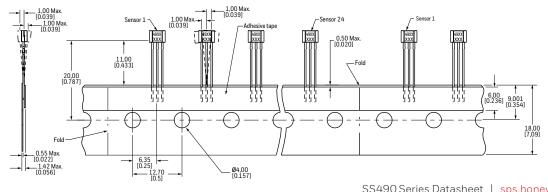
FIGURE 5. SS490 SERIES FLAT TO-92-STYLE MOUNTING AND DIMENSIONAL DRAWINGS (CONTINUED)
