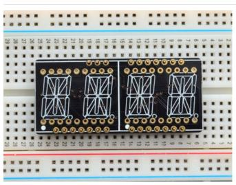
Add the FeatherWing PCB: Place the circuit board over the pins so that the short pins poke through the breakout pads
