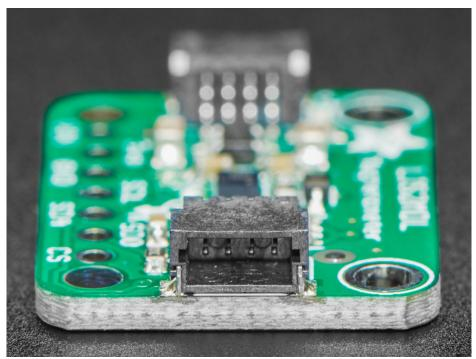
This adorable little magnetometer is quite capable but it is near-microscopic at 2mm square. To make things easier, we've put it on a breakout PCB along with support circuitry to let you use this little wonder with 3.3V (Feather/Raspberry Pi) or 5V (Arduino/ Metro328) logic levels.
