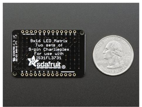
Pick up a driver board and your favorite color LEDs to match. You'll need to do some basic soldering to attach the driver backpack and matrix together, and run wires to your microcontroller, but its not too hard. Then install our Arduino code to get some LEDs blinking immediately. Our library is Adafruit\_GFX
