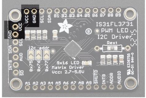
You can power the IS31 from 2.7-5.5VDC, but note that the same voltage is used for both power and logic. If you are using a **5V** logic device, just connect **VCC** to 5V.
