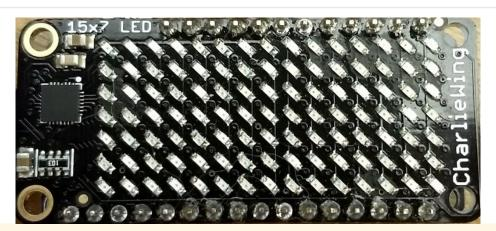
Be careful setting all pixels to 255 maximum brightness! This might pull more power than your computer's USB port can provide if you are powering your board over USB. Use an external powers supply or battery when lighting lots of LEDs to max brightness.
