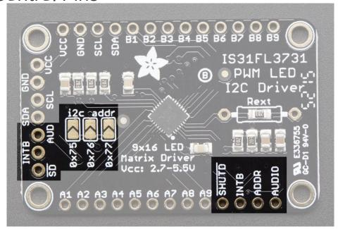
• SD - Shutdown pin, default pulled up to VCC. Connect to ground to put the chip in shutdown mode
