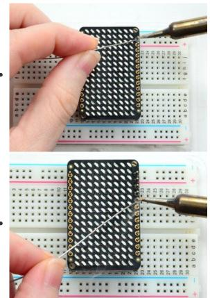
Solder in the two long header strips. Not all are connected on the LED matrix but it makes the connections mechanically stable.
