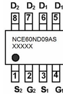
Marking and pin assignment
