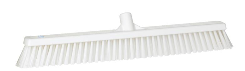
This sweeping broom has two types of bristles. When pushing the broom forward the front rows, which have firm bristles, loosen the dirt and push heavier debris. The softer bristles of the back rows, gather the finer particles. It is suitable for both wet and dry sweeping.
