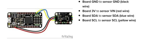
Or you can wire up the APDS9960 to your board exactly as shown on the previous pages for Arduino using an I2C connection. Here's an example of wiring a Feather M0 to the sensor with I2C:
