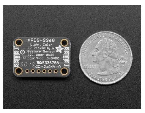
The APDS9960 from Avago Technologies has an integrated IR LED and driver, along with four directional photodiodes that sense reflected IR energy from the LED. It's proximity detection feature allows it to measure the distance an object is from the front of the sensor (up to a few centimeters) with 8 bit resolution.
