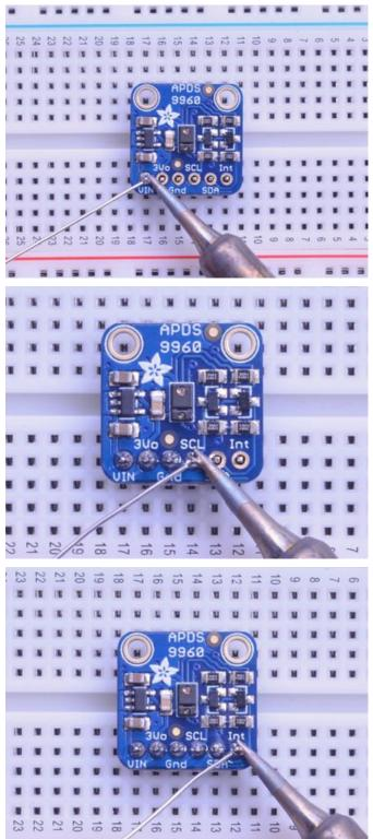
And Solder! Be sure to solder all 6 pins for reliable electrical contact.
