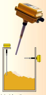
The CLS level switch is a microprocessor based, self calibrating level control with no moving parts, operating using the RF Capacitance principle.
