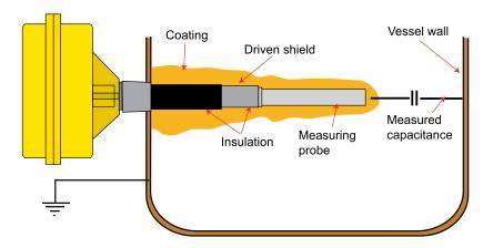
Simple capacitance probes operate by driving the probe to apply an RF signal between the stainless steel probe and the vessel wall. With the probe in free air, which has a dielectric value of 1.0, electronic circuitry measures the standing capacitance around the probe. When the air is displaced by material with a higher dielectric value the capacitance measured increases and an alarm can be triggered.
