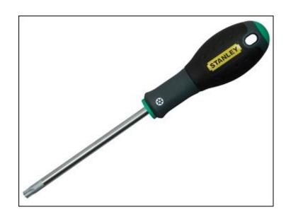
The Stanley FatMax Torx tip screwdrivers have a chrome vanadium steel bar which allows high torque and reduces the risk of tip breakage, and the handle is moulded directly to the shaft for a virtually unbreakable bond which gives long life and durability.
