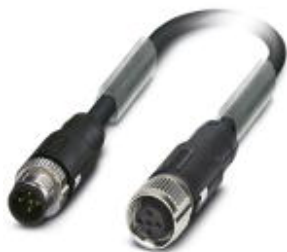
Sensor/Actuator cable, 5-position, PUR halogen-free, black-gray RAL 7021, shielded, Plug straight M12 SPEEDCON, B-coded, on Socket straight M12 SPEEDCON, B-coded, Cable length: 0.13 m
