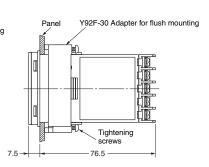
Note: 1. The recommended panel thickness is 1 to 4 mm.
