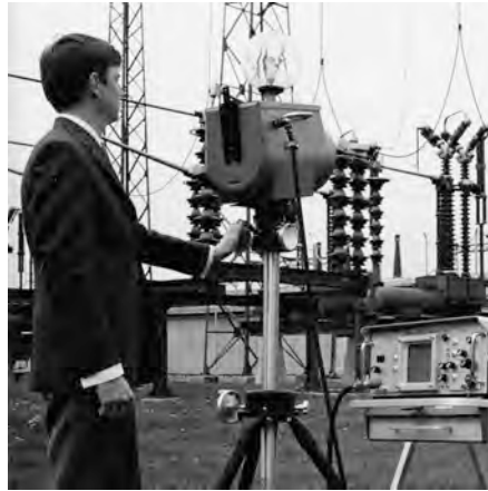
Figure 14.2 1969: Thermovision Model 661. The camera weighed approximately 25 kg (55 lb.), the oscilloscope 20 kg (44 lb.), and the tripod 15 kg (33 lb.). The operator also needed a 220 VAC generator set, and a 10 L (2.6 US gallon) jar with liquid nitrogen. To the left of the oscilloscope the Polaroid attachment (6 kg (13 lb.)) can be seen.
