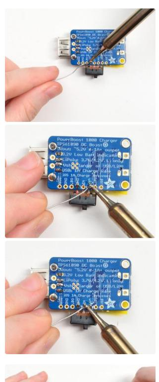
Solder in all three pins with any kind of solder making sure you have a good connection
