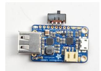
The switch will go into the breakout header, and attach to VS EN and GND The switch is symmetric so as long as those three pins are attached to the switch you are good to go
