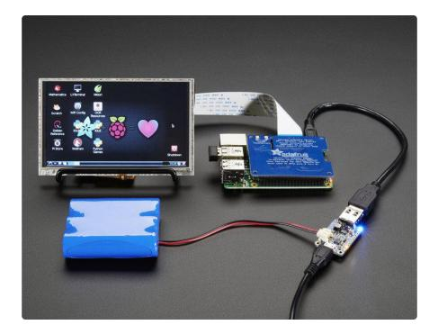
The PowerBoost 1000C has at the heart a <u>TPS61090 boost converter from TI (https://adafru.it/duQ)</u>. This boost converter chip has some really nice extras such as low battery detection, 2A internal switch, synchronous conversion, excellent efficiency, and 700KHz high-frequency operation. Check out these specs!
