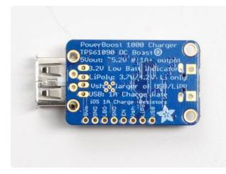
Snap the USB connector in so that all of the pins go through the PCB. Make sure you're solder them on the back of the PCB
