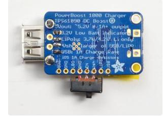
Flip over to solder the three pads in place
