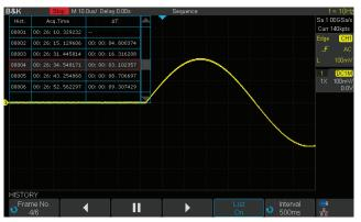
Segmented acquisition partitions the memory into multiple segments (up to 80,000) of the signal when trigger conditions are met. Recall stored segments using the History function.
