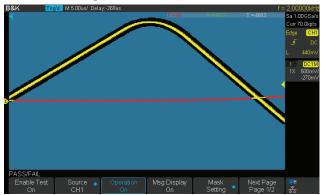
Generate a mask based on user defined parameters to identify pass/fail test results. Useful in long term signal monitoring or automated production line testing applications.
