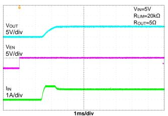
Figure 2. Turn-On Delay and Rise Time
