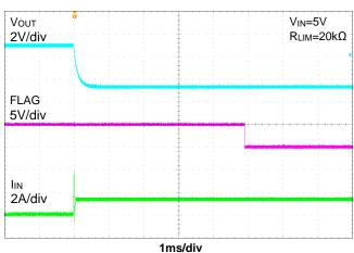
Figure 5. No Load to 1Ω Transient Response
