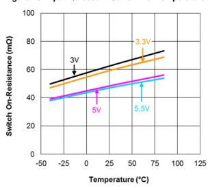
Figure 12. Switch On-Resistance vs. Temperature
