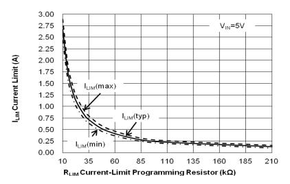
Figure 14. Current-Limit Threshold vs. RLIM
