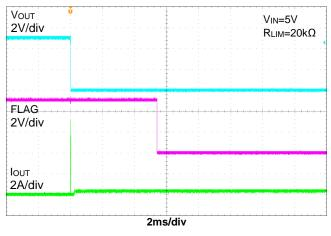
Figure 6. Short-Circuit Current Limit Response
