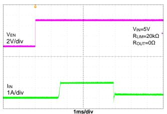
Figure 4. Device Enabled into Short-Circuit
