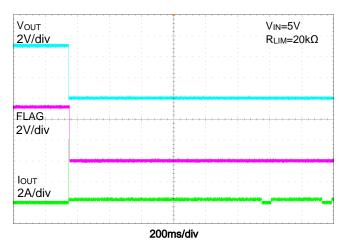
Figure 7. Extended Short-Circuit into Thermal Cycles
