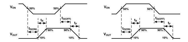
Figure 1. Voltage Waveforms: AP22652/52A (Left), AP22653/53A (Right)
