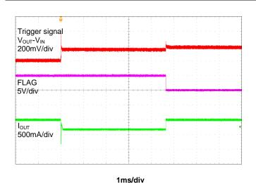
Figure 8. Reverse Current Limit Response
