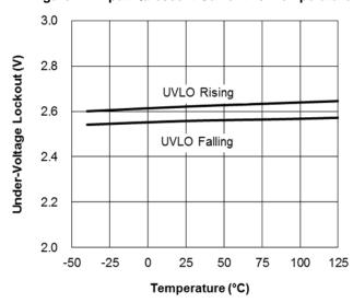
Figure 13. Under-Voltage Lock Out vs. Temperature
