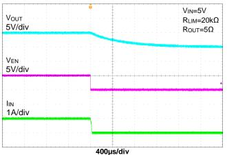
Figure 3. Turn-Off Delay and Fall Time
