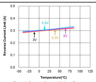
Figure 9. Reverse Current Limit vs. Temperature
