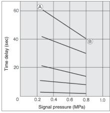
Example) (A) is the point, which is set by the input signal pressure 0.25 MPa, with a delay time of 60 sec. With the same status, if the input signal pressure is increased to 0.8 MPa, the delay time varies to the  $\ensuremath{\mathbb{B}}$  point (≅ 40 sec).
