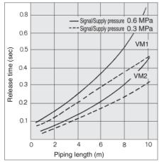
If the input signal (PIL) is turned OFF, the release time of the time delay valve changes depending upon the effective area of the valve and the length of piping. Please refer to the above graph for the standard values.
