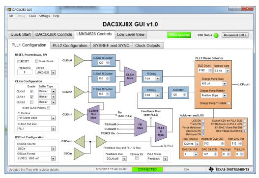
Figure 4. LMK04828 Controls Tab
