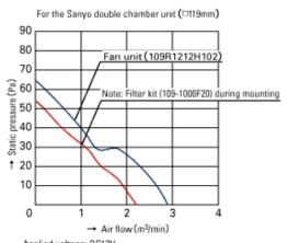
Applied voltage: DC12V Note: Measuring with the fan suction side-fitted filter kit
