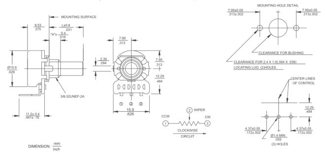
Series 275X Metal Shaft, Bushing Mount, Printed Circuit "X" Type Terminals
