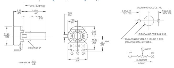
Series 270T-2 Dual Section, Metal Shaft, Bushing Mount, Solder Lug "T" Type Terminals
