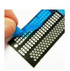
**Assembly:** Before using your breakout board you will need to solder the edge connector into place on the PCB.
