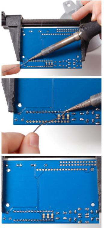
Flip over the PCB and solder in the 28 pins of the port expander.
