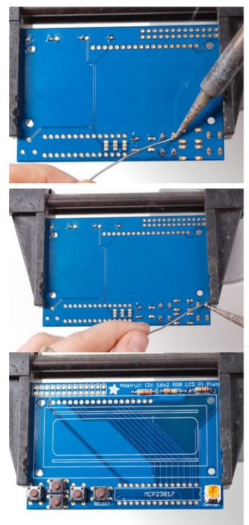
Next, place the 10K potentiometer (the orange-faced thing with three legs) into the spot above the RESET button. It will only fit one way. This is the contrast potentiometer which will adjust how dark the characters appear. All displays are slightly different so you'll adjust this once the display is soldered in.
