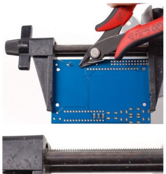
Once the soldering is complete, we can clean up by clipping the leads of the resistor. This keeps them from shorting to something else. Use diagonal or flush cutters to clip the wires right above where the solder joint ends.
