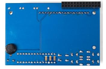
WARNING: If you're using the new Raspberry Pi model B+ with 4 USB ports you will need to take some extra steps to ensure the backlight resistor leads do not touch the USB ports and short out. See the steps below for more details.
