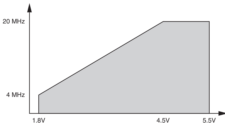
Figure 18-1. Maximum Frequency vs. V_{CC}
