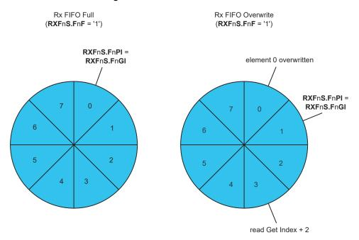
After reading from the Rx FIFO, the number of the last element read has to be written to the Rx FIFO Acknowledge Index RXFnA.FnA. This increments the get index to that element number. In case the put index has not been incremented to this Rx FIFO element, the Rx FIFO full condition is reset (RXFnS.FnF = '0').
