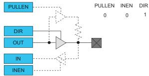
Figure 28-7. I/O Configuration - Totem-Pole Output with Enabled Input
