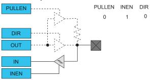
Figure 28-5. I/O Configuration - Input with Pull
