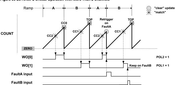
Figure 36-20. RAMP2 Critical Operation With More Than 2 Channels
