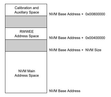
The lower rows in the NVM main address space can be allocated as a boot loader section by using the NVM User Row BOOTPROT fuses, and the upper rows can be allocated to EEPROM Emulation section by using the NVM User Row EEPROM Size fuses, as shown in the figure below.
