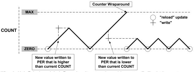
When double buffering is used, the buffer can be written at any time and the counter will still maintain correct operation. The period register is always updated on the update condition, as shown in Figure 36-13. This prevents wraparound and the generation of odd waveforms.
