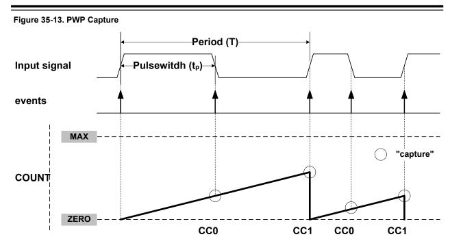
Selecting PWP in the Event Action bit group in the Event Control register (EVCTRL.EVACT) enables the TC to perform one capture action on the rising edge and another one on the falling edge. The period T will be captured into CC1 and the pulse width  $t_p$  in CC0. EVCTRL.EVACT = PPW (period and pulse-width) offers identical functionality, but will capture T into CC0 and  $t_p$  into CC1.
