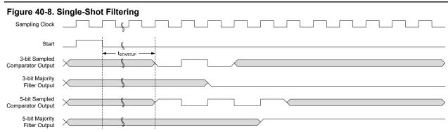
During sleep modes, filtering is supported only for single-shot measurements. Filtering must be disabled if continuous measurements will be done during sleep modes, or the resulting interrupt/event may be generated incorrectly.
