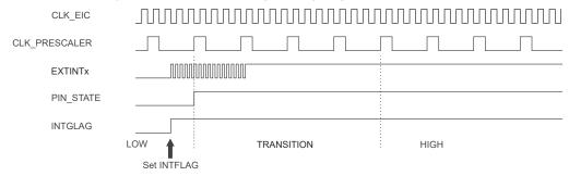
In this mode, the EIC clock is requested. The asynchronous Edge Detection mode can be used in Idle and Standby Sleep modes.
