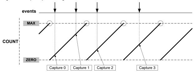
For input capture, the buffer register and the corresponding CCx act like a FIFO. When CCx is empty or read, any content in CCBUFx is transferred to CCx. The buffer valid flag is passed to set the CCx interrupt flag (IF) and generate the optional interrupt, event or DMA request. CCBUFx register value can't be read, all captured data must be read from CCx register.
