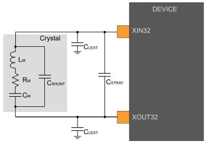
The user must choose a crystal oscillator where the crystal load capacitance C<sub>L</sub> is within the range given in the table. The exact value of CL can be found in the crystal data sheet. The capacitance of the external capacitors (CLEXT) can then be computed as follows:
