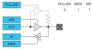
Figure 28-8. I/O Configuration - Output with Pull
