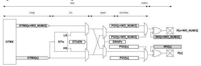
The output matrix (OTMX) unit distributes compare channels, according to the selectable configurations in Table 36-4.
