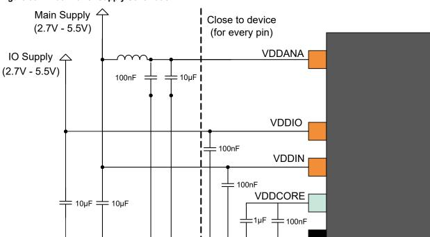
Figure 53-2. Dual Power Supply Schematic
