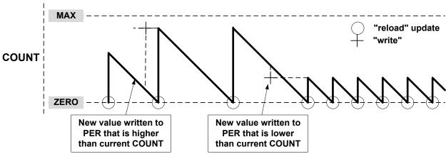
A counter wraparound can occur in any operation mode when up-counting without buffering, see Figure 36-10. COUNT and TOP are continuously compared, so when a new value that is lower than the current COUNT is written to TOP, COUNT will wrap before a compare match.
