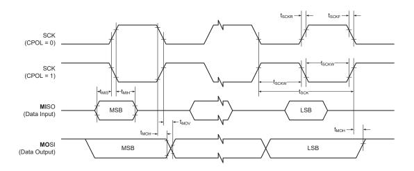
Figure 45-8. SPI Timing Requirements in Client Mode
