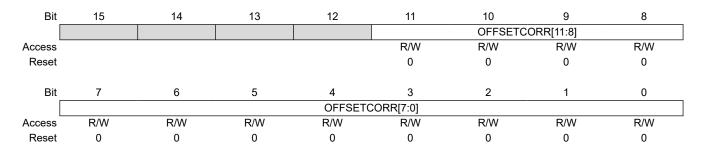
Bits 11:0 - OFFSETCORR[11:0] Offset Correction Value
