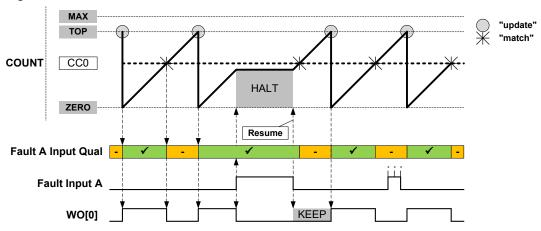
Figure 36-31. Waveform Generation with Fault Qualification, Halt, and Restart Actions
