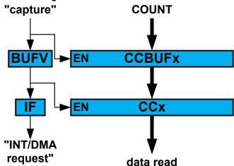
The TCC can detect capture overflow of the input capture channels: When a new capture event is detected while the Capture Buffer Valid flag (STATUS.CCBUFV) is still set, the new timestamp will not be stored and INTFLAG.ERR will
