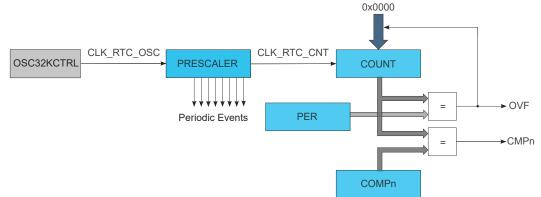
Figure 24-3. RTC Block Diagram (Mode 2 — Clock/Calendar)
