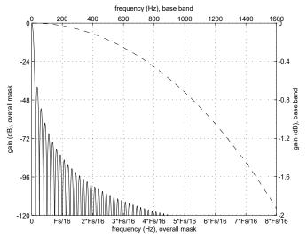
The zeros of this filter are located at multiples of CLK\_SDADC\_FS/128.
