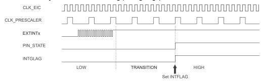
In the Synchronous Edge Detection mode, the EIC clock is required. The Synchronous Edge Detection mode can be used in Idle and Standby Sleep modes.
