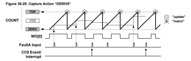
This is configured by writing 0x1 to the Fault n Halt mode bits in the Recoverable Fault n Configuration register (FCTRLn.HALT). When enabled, the timer/counter is halted and the cycle is extended as long as the corresponding fault is present.
