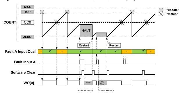
Figure 36-32. Waveform Generation with Software Halt, Fault Qualification, Keep and Restart Actions
