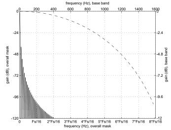
The zeros of this filter are located at multiples of CLK SDADC FS/256.
