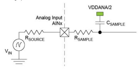
The minimum sampling time  $t_{\text{samplehold}}$  for a given  $R_{\text{source}}$  can be calculated using this formula:
