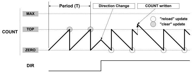
Due to asynchronous clock domains, the internal counter settings are written when the synchronization is complete. Normal operation must be used when using the counter as timer base for the capture channels.
