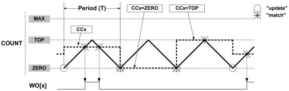
Using dual-slope PWM results in a lower maximum operation frequency compared to single-slope PWM generation. The period (TOP) defines the PWM resolution. The minimum resolution is 1 bit (TOP=0x00000001).
