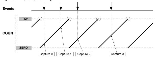
The TC can detect capture overflow of the input capture channels: When a new capture event is detected while the Capture Interrupt flag (INTFLAG.MCx) is still set, the new timestamp will not be stored and INTFLAG.ERR will be set.
