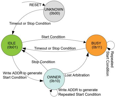
The Bus state machine is active when the I<sup>2</sup>C host is enabled.
