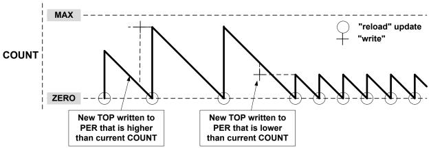
When double buffering is used, the buffer can be written at any time and the counter will still maintain correct operation. The period register is always updated on the update condition, as shown in Figure 35-10. This prevents wraparound and the generation of odd waveforms.
