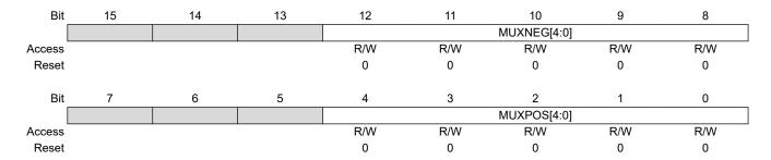
Bits 12:8 - MUXNEG[4:0] Negative MUX Input Selection
