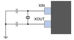
The crystal must be located as close to the device as possible. Long-signal lines may cause too high of a load to operate the crystal, and cause crosstalk to other parts of the system.
