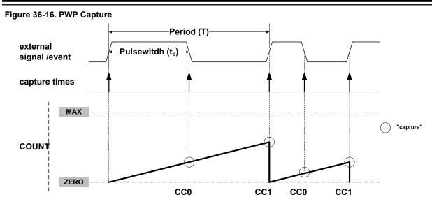
Selecting PWP or PPW in the Timer/Counter Event Input 1 Action bit group in the Event Control register (EVCTRL.EVACT1) enables the TCC to perform one capture action on the rising edge and the other one on the falling edge. When using PPW (period and pulse-width) event action, period T will be captured into CC0 and the pulse-width to into CC1. The PWP (Pulse-width and Period) event action offers the same functionality, but T will be captured into CC1 and  $t_p$  into CC0.
