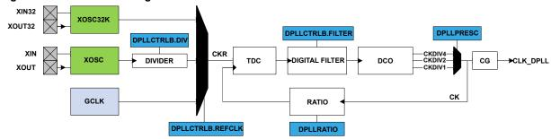
When the controller is disabled, the output clock is low. If the Loop Divider Ratio Fractional part bit field in the DPLL Ratio register (DPLLRATIO.LDRFRAC) is zero, the DPLL works in integer mode. Otherwise, the fractional mode is activated. Note that the fractional part has a negative impact on the jitter of the DPLL.
