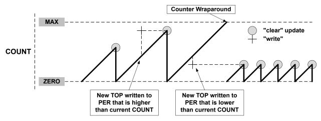
A counter wraparound can occur in any operation mode when up-counting without buffering, see Figure 35-8.
