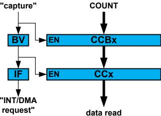
For input capture, the buffer register and the corresponding CCx act like a FIFO. When CCx is empty or read, any content in CCBUFx is transferred to CCx. The buffer valid flag is passed to set the CCx interrupt flag (IF) and generate the optional interrupt, event, or DMA request. The CCBUFx register value can't be read, all captured data must be read from CCx register.
