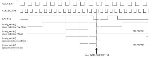
Detection latency depends on the detection mode.
