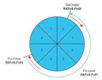
When reading from an Rx FIFO, Rx FIFO Get Index RXFnS.FnGI • FIFO Element Size has to be added to the corresponding Rx FIFO start address RXFnC.FnSA.
