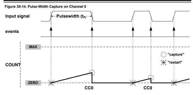
The TC can detect capture overflow of the input capture channels: When a new capture event is detected while the Capture Interrupt flag (INTFLAG.MCx) is still set, the new timestamp will not be stored and INTFLAG.ERR will be set.
