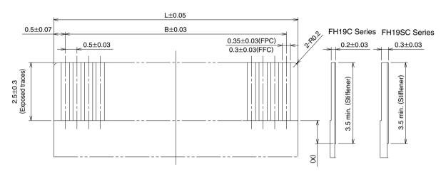
Note 1: Stiffener dimension should be 3.5mm min., and X dimension should be 0.5mm for improved flexibility of FPC.
