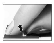
2) Assure that the FPC/FFC is fully inserted parallel to mounting surface, with the exposed conductive traces facing down.
