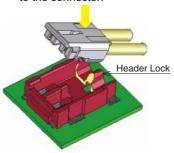
(2) Then, in a slight, rotating movement, push the front section of the plug down.
