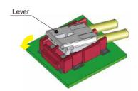
(3) Keep pressing down until a "click" feeling is sensed. The connector is now fully and properly mated.
