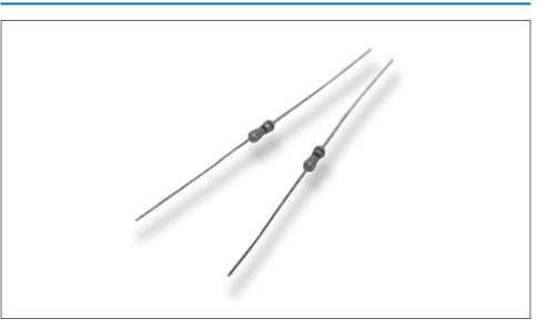
Metal glaze resistors are manufactured using thick film techniques. The ceramic slugs have the thick film applied, the film is fired and end caps are forced onto the slugs, the resistive element is spiralled to value and lead wires are welded onto the end caps. Four layers of coating are applied - the first being a phenolic resin, the other three being epoxy.
