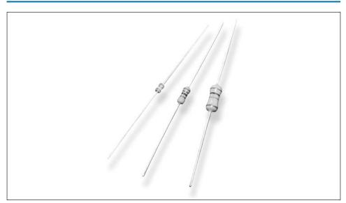
The resistive element comprises a thin film of nickel-chrome alloy evaporated onto a high thermal conductivity ceramic element. Metal end caps are force fitted to the element prior to spiralling to value. Tinned copper lead wires are welded to the end caps and the components are then coated. One coat of phenolic resin is followed by three coats of epoxy resin. All resistors are tested for value and tolerance.
