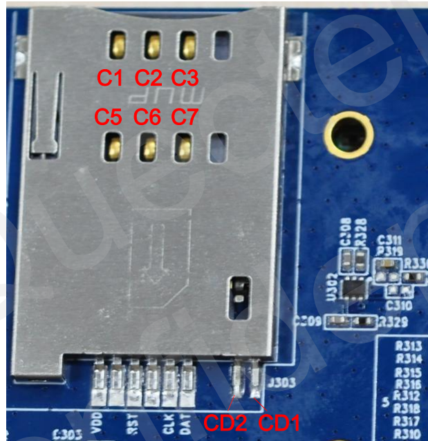
Figure 16: Pins Assignment of USIM Card Holder
