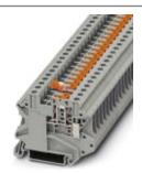
Knife disconnect terminal block, nom. voltage: 500 V, nominal current: 20 A, connection method: Screw connection, cross section: 0.14 mm² - 6 mm², AWG: 26 - 10, length: 57.8 mm, width: 6.2 mm, color: gray, mounting: NS 35/7,5, NS 35/15
