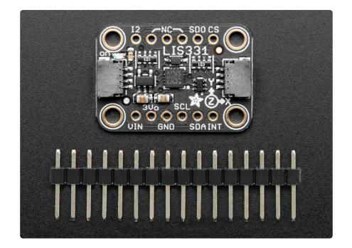
In addition to their substantial measurement capability, the LIS331s have built in and c onfigurable high-pass and low-pass filters to adjust the readings to your application. Adjustable data rates also allow you to adjust how frequently to take measurements depending on your power budget, and SPI and I2C interfaces give them flexibility to allow them to be used in a range of applications.
