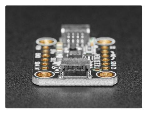
The breakout for the LIS331 family takes one of these little dynamos and puts it on a custom made PCB in the <u>STEMMA QT form factor</u> (https://adafru.it/LBQ), making them easy to interface with. The <u>STEMMA QT connectors</u> (https://adafru.it/JqB) on either side are compatible with the <u>SparkFun Qwiic</u> (https://adafru.it/Fpw) I2C connectors. This allows you to make solderless connections between your development board
