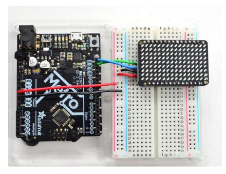
You can easily wire this breakout to any microcontroller, we'll be using an Arduino. For another kind of microcontroller, as long as you have I2C pins available, just check out the library, then port the code.
