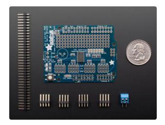
Check you have everything you need: assembled shield PCB, 0.1" male header, 4 of 3x4 male header, and a 2 pin terminal block
