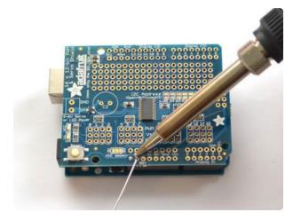
Solder each of the pins to secure the shield to the headers
