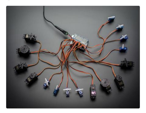
Driving servo motors with the Arduino Servo library is pretty easy, but each one consumes a precious pin - not to mention some Arduino processing power. The Adafruit 16-Channel 12-bit PWM/Servo Driver Shield will drive up to 16 servos over I2C with only 2 pins. The on-board PWM controller will drive all 16 channels simultaneously with no additional Arduino processing overhead. What's more, you can stack up to 62 of them to control even more servos - all with the same 2 pins!
