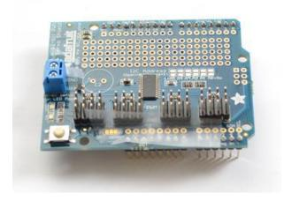
Flip the board over and solder the terminal block
