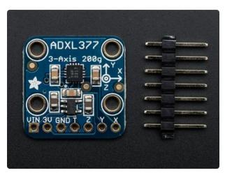
The ADXL377 can measure at least +/-200G(!) in the X, Y and Z axis. This is the sensor for measuring extreme dynamic accelerations encountered in applications such as rocketry experiments and high-impact shock measurements.
