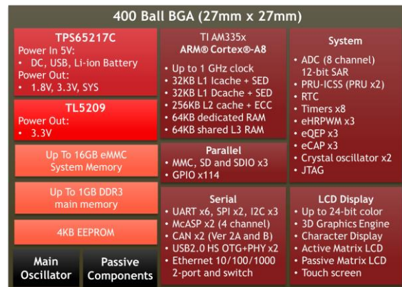
OSD335x C-SiP Block Diagram
