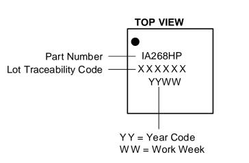
Figure 15. Part Number Package Marking
