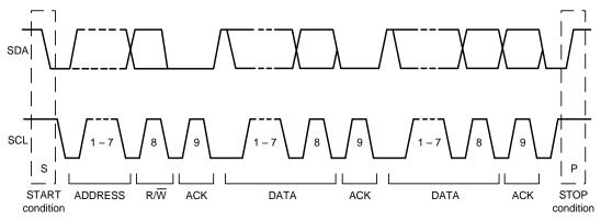
Figure 10. Complete I<sup>2</sup>C Data Transfer
