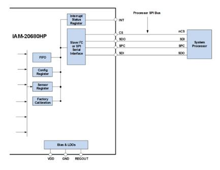
Figure 7. IAM-20680HP Solution Using SPI Interface
