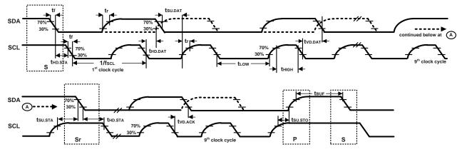
Figure 1. I<sup>2</sup>C Bus Timing Diagram
