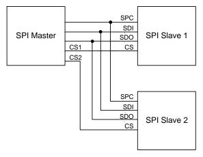
Figure 11. Typical SPI Master/Slave Configuration
