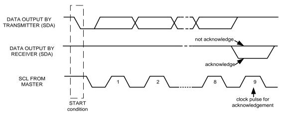
Figure 9. Acknowledge on the I<sup>2</sup>C Bus
