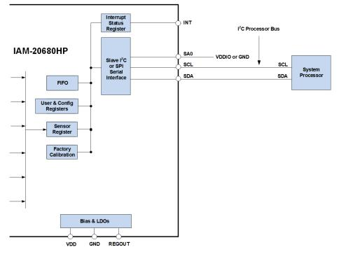
Figure 6. IAM-20680HP Solution Using I<sup>2</sup>C Interface
