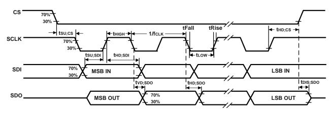
Figure 2. SPI Bus Timing Diagram
