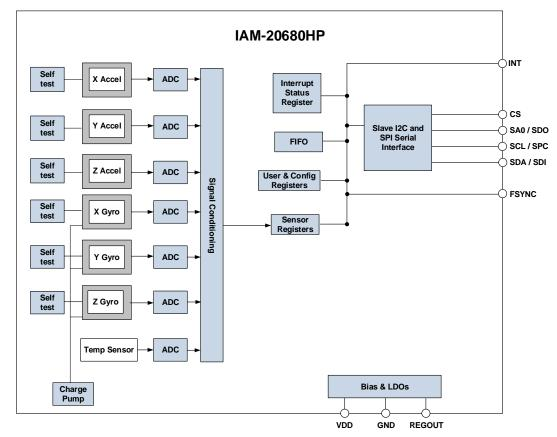
Figure 5. IAM-20680HP Block Diagram
