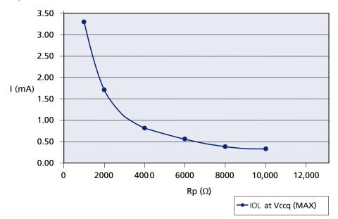
Figure 32: IOL vs Rp (V<sub>CCQ</sub> = 1.7-1.95V)
