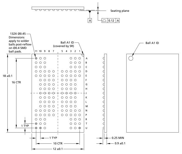
Notes: 1. All dimensions are in millimeters.2. Solder ball material: SAC305 (96.5% Sn, 3% Ag, 0.5% Cu).
