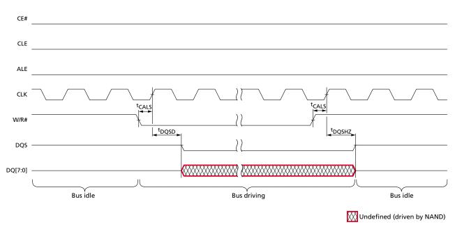
Note: 1. Only the selected die (LUN) drives DQS and DQ[7:0]. During an interleaved die (multi-LUN) operation, the host must use the READ STATUS ENHANCED (78h) to prevent data output contention.
