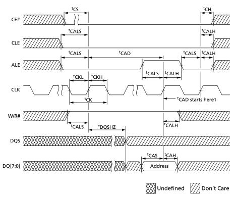
Note: 1. When CE# remains LOW, <sup>t</sup>CAD begins at the rising edge of the clock from which the command cycle is latched for subsequent command, address, data input, or data output cycle(s).
