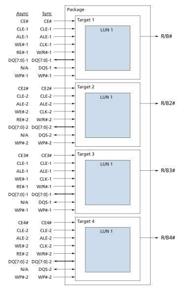
Note: 1. LGA devices do not support the synchronous interface.
