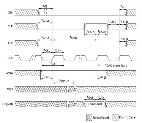
Note: 1. When CE# remains LOW, <sup>t</sup>CAD begins at the rising edge of the clock from which the command cycle is latched for subsequent command, address, data input, or data output cycle(s).
