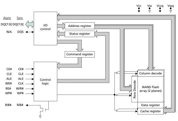
Notes: 1. N/A: This signal is tri-stated when the asynchronous interface is active.2. Some devices do not include the synchronous interface.
