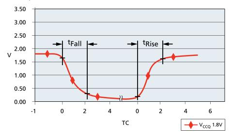
Notes: 1. <sup>t</sup>FALL is  $V_{OH(DC)}$  to  $V_{OL(AC)}$  and <sup>t</sup>RISE is  $V_{OL(DC)}$  to  $V_{OH(AC)}$ .
