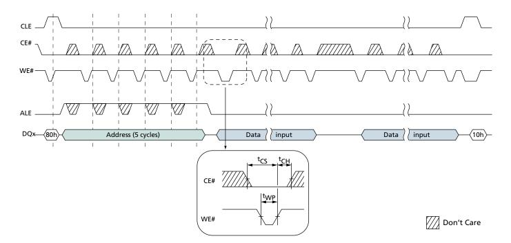
Figure 91: PROGRAM PAGE Operation with CHANGE WRITE COLUMN
