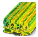
Ground modular terminal block, number of connections: 4, connection method: Push-in connection, 1 level, cross section:  $0.5~\text{mm}^2$  -  $10~\text{mm}^2$ , mounting type: NS 35/7,5, NS 35/15, color: green-yellow
