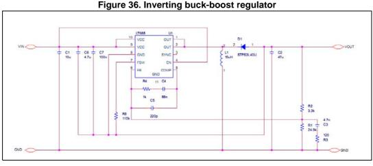
The GND pin of the device is connected to the output voltage so, given the output voltage, the input voltage range is limited by the maximum voltage the device can withstand across
