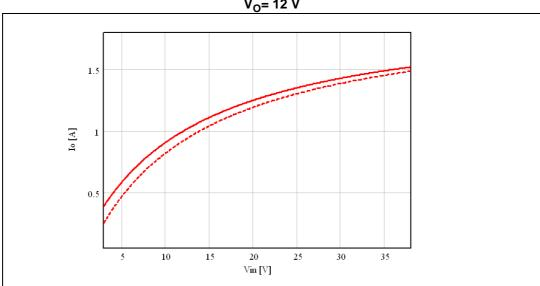
Figure 35. Maximum output current according to max. DC switch current (2.0 A):  $V_{O}$ = 12 V
