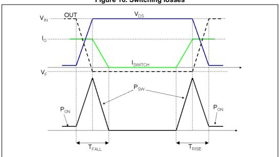
Figure 16. Switching losses
