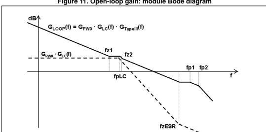
Figure 11. Open-loop gain: module Bode diagram
