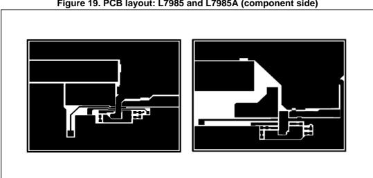
Figure 19. PCB layout: L7985 and L7985A (component side)
