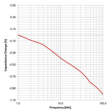
Test Equipment: E4991A or equivalent
