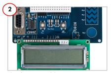
Plug the LCD module into port P8.
