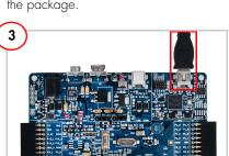
Plug the USB cable into your PC and the onboard programming USB port (11).
