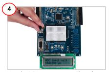
Vary the R56 potentiometer. The voltage is displayed with a 20-bit resolution on the LCD module.
