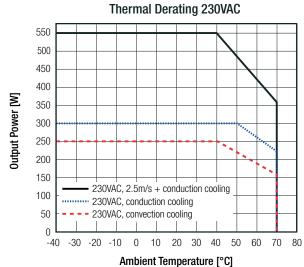
Conduction Cooling: ground plane ref.: 2mm alloy; size A4
