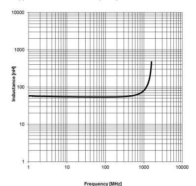
DESCRIPTION Projection **WE-CAIR Air coil** Würth Elektronik eiSos GmbH & Co. KG EMC & Inductive Solutions Max-Eyth-Str. 1 Order.- No. 74638 Waldenburg COMPLIANT SIZE Germany Tel. +49 (0) 79 42 945 - 0 744912156 www.we-online.com A4 2014-03-24 SSt 1.0 HBH eiSos@we-online.com REV BY Size: 4248 DATE CHECKED
