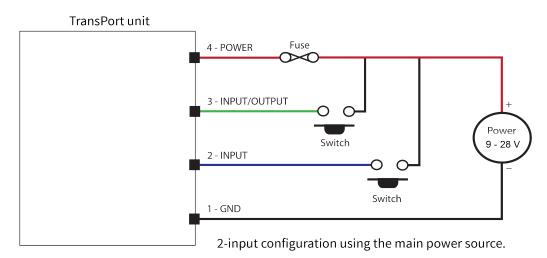
The supply voltage is limited by the maximum allowed 28 V of the inputs.
