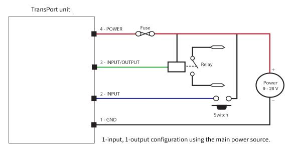
The supply voltage is limited by the maximum allowed 28 V or the I/O lines.
