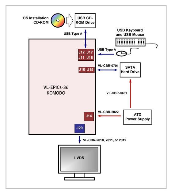
Figure 2. Typical Start-up Configuration
