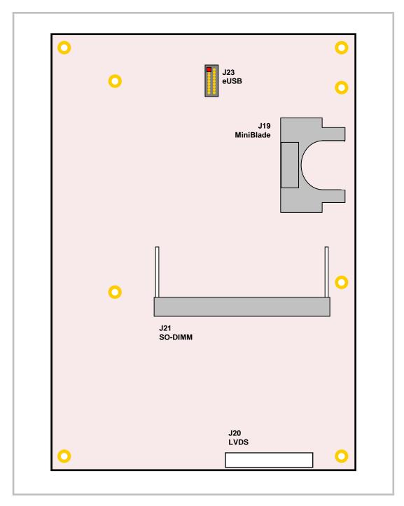
Figure 7. Connector Locations (Bottom)
