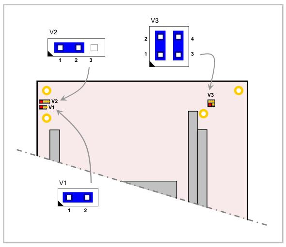
Figure 9. Jumper Block Locations
