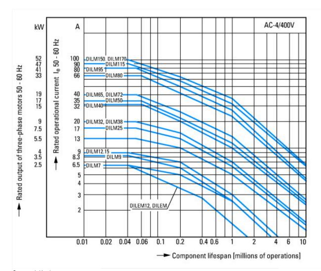
Extreme switching duty Squirrel-cage motor Operating characteristics Inching, plugging, reversing Electrical characteristics Make: up to 6 x rated motor current Break: up to 6 x rated motor current Utilization category 100 % AC-4 Typical applications Printing presses Wire-drawing machines Centrifuges
