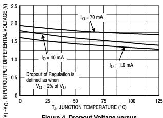
Figure 4. Dropout Voltage versus Junction Temperature
