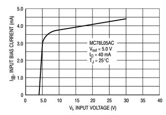
Figure 6. Input Bias Current versus Input Voltage
