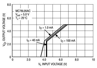
Figure 3. Dropout Characteristics
