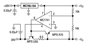
Figure 10. ±15 V Tracking Voltage Regulator
