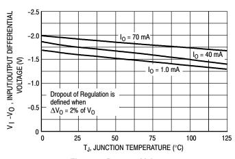
Figure 5. Dropout Voltage versus Junction Temperature
