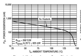
Figure 8. Maximum Average Power Dissipation versus Ambient Temperature (TO-92)
