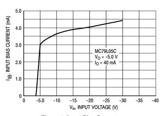
Figure 7. Input Bias Current versus Input Voltage
