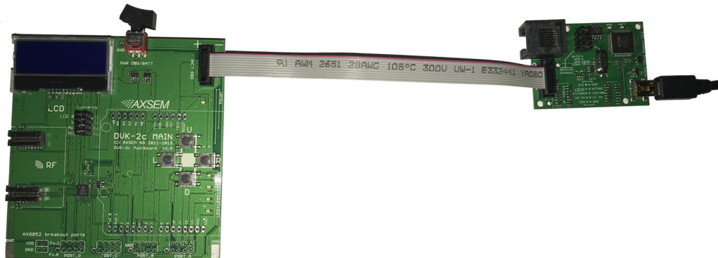
Figure 3. DVK-2 Main Board Connected to the AXDBG
